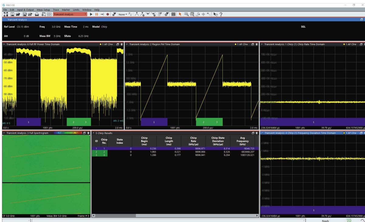
Fig. 4: Transient analysis of a chirp sequence signal with the R&S®VSE-K60c transient analysis option. The pulse power versus time is shown at the top left. The linear frequency response can be seen in the top middle and in the spectrogram on the bottom left. The software lists the properties of the detected pulses in a table (bottom middle). The properties can also be investigated in detail in graphical form. The chirp rate and frequency deviation are shown on the right.
