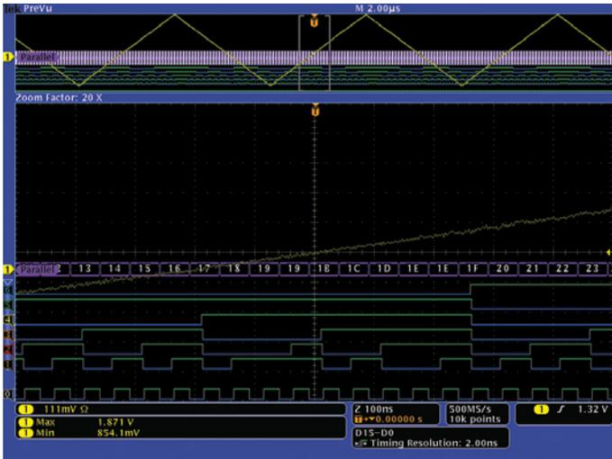
**Figure 24.** The MSO triggered on the rising edge of the input to the ADC and Wave Inspector zooms in so that parallel bus decode hex values are easily seen. The test ramp signal is on channel one. At the bottom of the display is the ADC clock on digital channel zero. The ADC digital output bus signals one through six are above the clock waveform. The ADC digital signals are grouped together into the clocked parallel bus at the center of the display.
