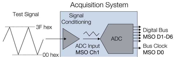
Figure 23. Verify sensor data acquisition system output range.
