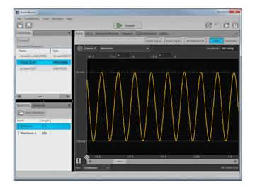
The Tektronix AWG5200 series features a digital complex modulator and multi-rate interpolation. With this internal IQ modulation feature, you remove the IQ mismatches that are attributed to external modulators and mixers. Also with this modulator, there is no in-band carrier feed-through, and there are no images. With its built in interpolators, it also affords the ability to create waveforms most efficiently reducing waveform size and compilation times as well as extending playback time.
